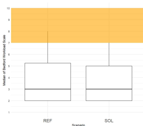
Figure 64. Median values of the Bedford Workload Scale, separated into the reference scenario (current MergeStrip) and the solution scenario (new MergeStrip, what-if function).
