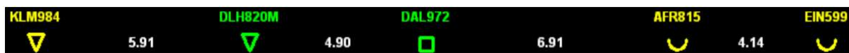
Figure 9. The Centerline Separation Visualization Tool. The symbols mark the position of aircraft (triangle), ghosts (square) and TargetWindows (semicircle). The label colors represent the aircraft weight class (yellow: medium; green: heavy) and the white numbers between the labels indicate the current separation between them.
