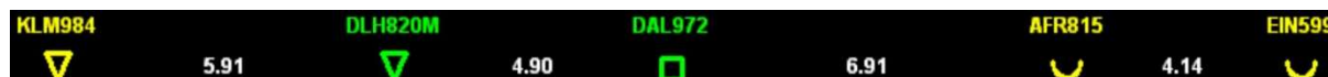
Figure 8: Detail extract of the Final Distance Indicator with the actual separation between aircraft on a final.
