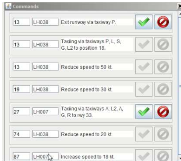
Figure 4-16: TRACC Display - possible configuration of Advisory Panel. Each row represents a suggested clearance. The controller can validate or discard the clearance using the two available buttons. For each clearance, the remaining time, callsign and a description of the instruction are provided, only one clearance per aircraft is active at the same time. The other ones are grayed and therefore inactive.
