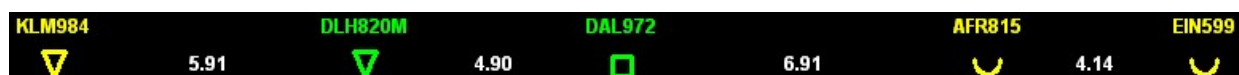
Figure 4-3: The Centerline Separation Visualization Tool. The symbols mark the position of aircraft (triangle), ghosts (square) and TargetWindows (semicircle). The label colors represent the aircraft weight class (yellow: medium; green: heavy) and the white numbers between the labels indicate the current separation between them.
