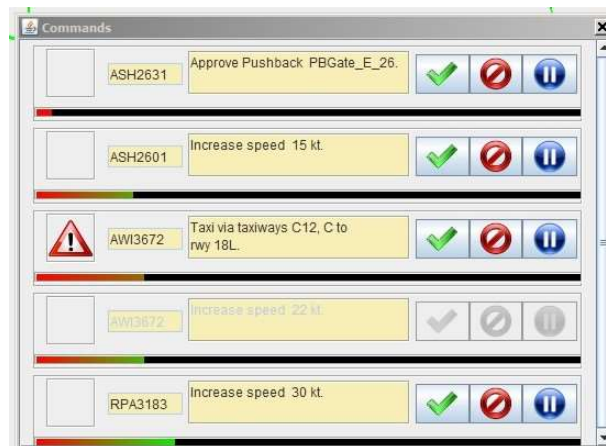
Figure 4-17: TRACC Display - possible configuration of Advisory Panel. Each row represents a suggested clearance. The controller can validate, discard or pause a clearance using the three available buttons. For each clearance, a timer, the callsign and a description of the instruction are provided. Only one clearance per aircraft is active at the same time. The other ones are grayed. The most urgent instruction to be issued is highlighted through an alert symbol.
