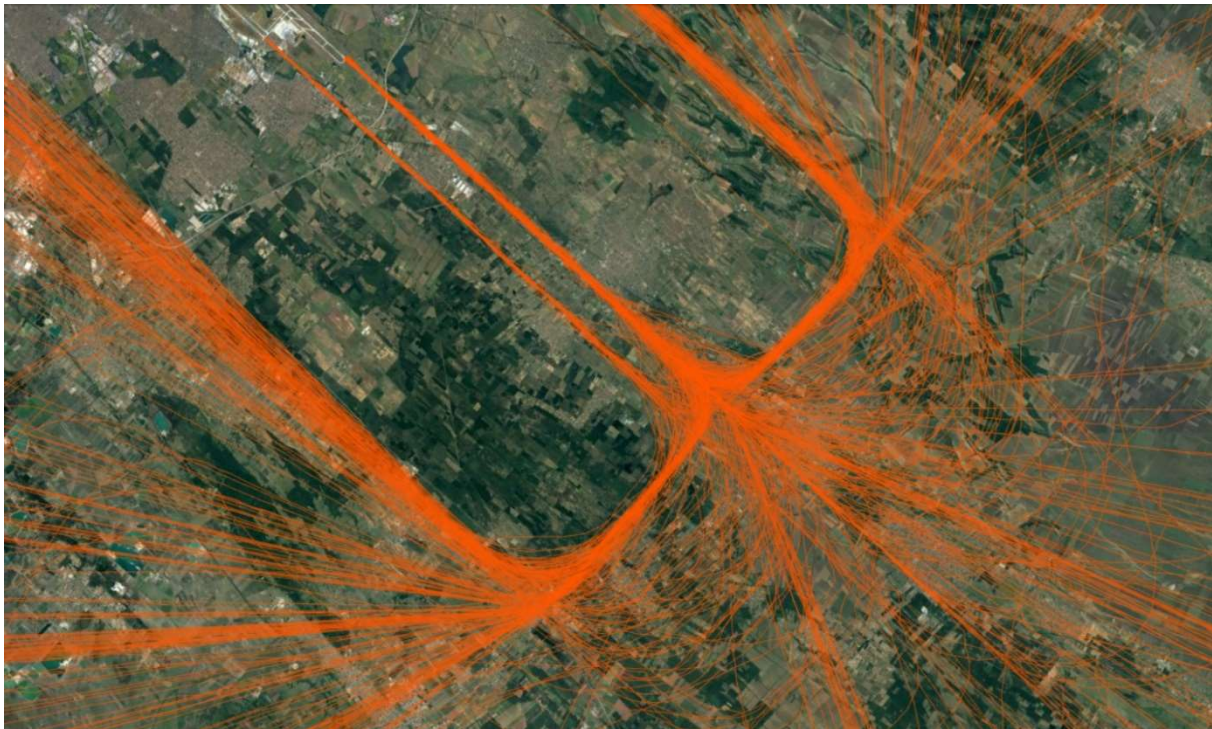
Figure 5-2: T-Bar based Instrument Approach – Aircraft flight path as deduced from real radar data.
