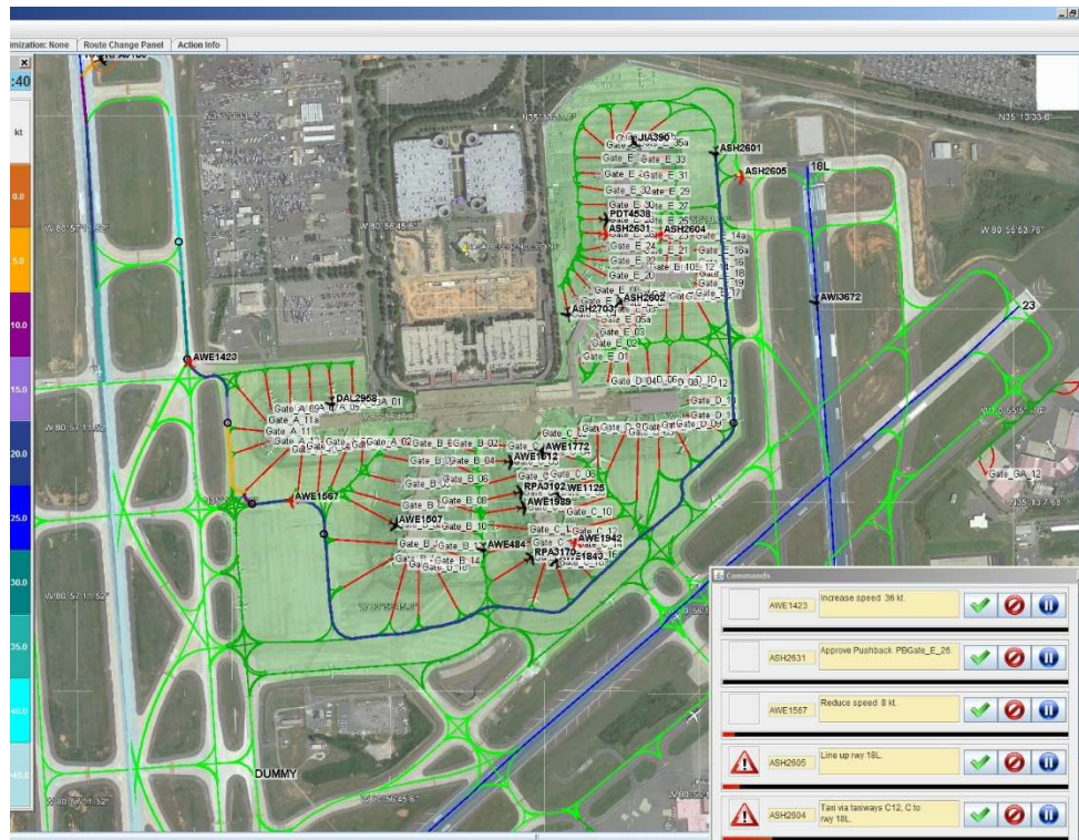
Figure 4-18: TRACC’s Traffic situation display with advisory panel and the overview of trajectory colors assigned to taxi speeds at the left border.
